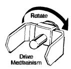
If bin does not go all the way back, remove it and rotate the drive mechanism 1/4 turn. Then push bin back again until the tab on the bin locks into the slot in the shelf.
